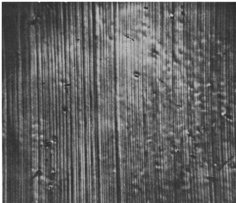
FIG. 17.33 Twinned structure (tetragonal) in an indium-thallium alloy after transformation. (Burkart, M. W., and Read, T. A., Trans. AIME , 197 1516 [1953].)
