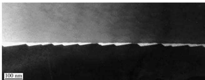
**FIGURE 29.9.** Diffuse-scatter DF image of a glassy material at a GB in a bicrystal of  $\text{Al}_2\text{O}_3$ .
