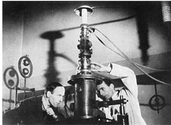
**FIGURE 1.1.** The electron microscope built by Ruska (in the lab coat) and Knoll, in Berlin in the early 1930s.
