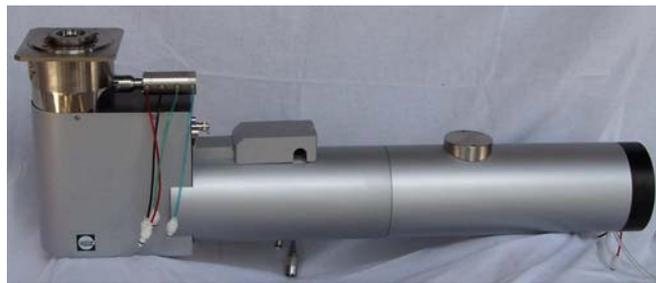
**FIGURE 37.3.** A Gatan Tridiem PEELS which interfaces below the viewing screen of an AEM.
