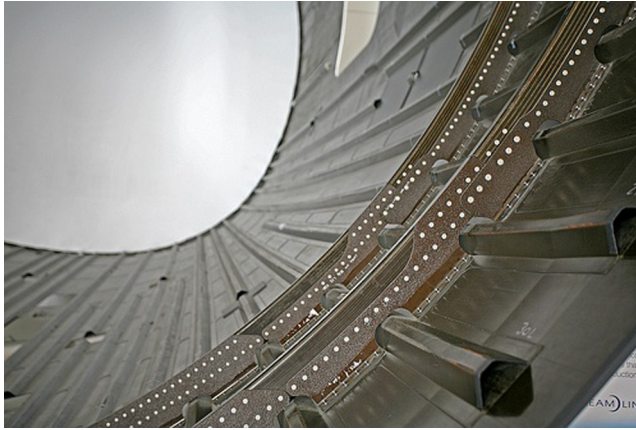
Figure 1.6 A typical modern carbon fibre/epoxy fuselage section.
