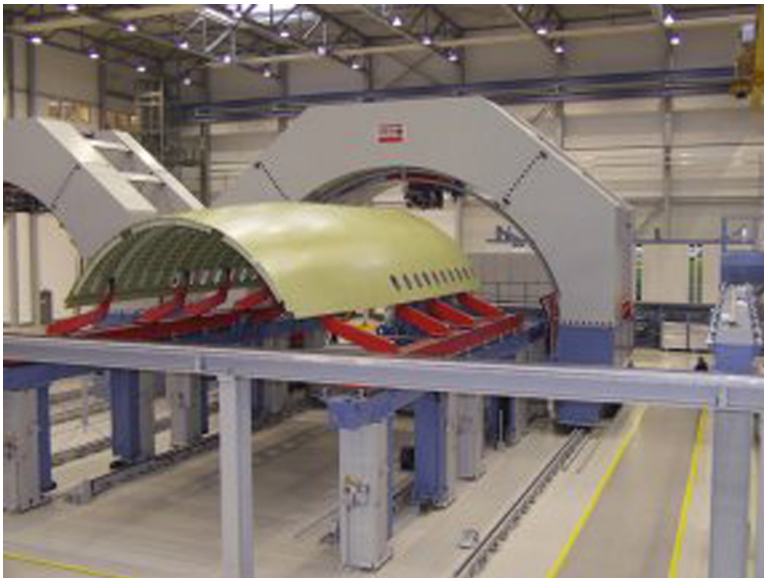
Figure 1.5 A380 Glare fuselage crown. Courtesy of Airbus S.A.S.
