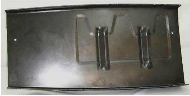
Figure 1.4 A typical aircraft composite wing rib element produced by RTM. Courtesy of Polyworx, RTM-Worx.
