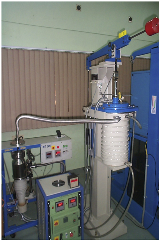
Fig. 2. Impression creep testing machine.
