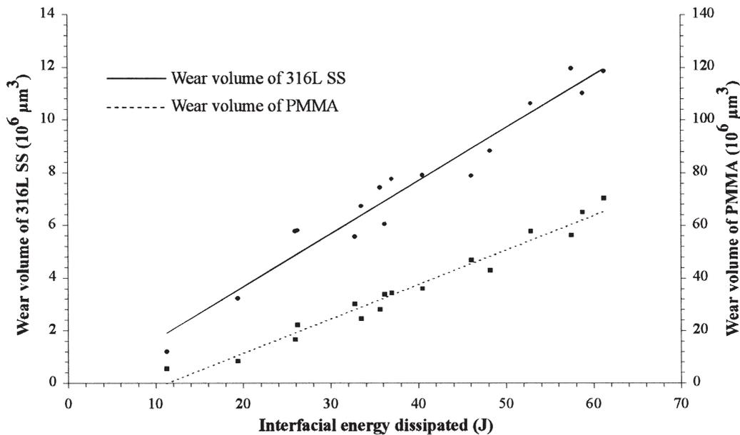
Fig. 10. Wear volume of 316L SS and PMMA as a function of total interfacial energy dissipated in the contact. Tests performed in Ringer's solution.
