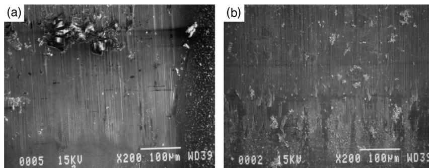
Fig. 3. SEM observation of wear surfaces (frequency 1 Hz, displacement ±40 µm, normal force 4 N/mm, duration of test 20,000 cycles, Ringer's solution). (a) View of surface of 316L SS. (b) View of surface of PMMA.
