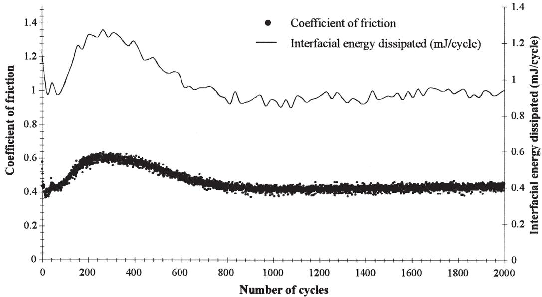
Fig. 9. Combined evolution of coefficient of friction and interfacial energy dissipated per cycle. Contact PMMA Ø20/316L SS plane in Ringer's solution. Frequency 1 Hz, displacement  $\pm 40 \mu\text{m}$ , normal force 1.5 N/mm.
