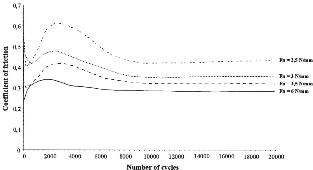
Fig. 6. Coefficient of friction as a function of normal force applied. Contact PMMA Ø20/316L SS plane in Ringer's solution. Frequency, 1 Hz, displacement  $\pm 40$   $\mu\text{m}$ , 20,000 cycles of fretting.
