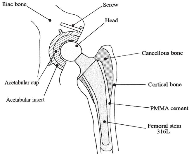
Fig. 1. Diagram showing cemented implantation of a total hip joint prosthesis.
