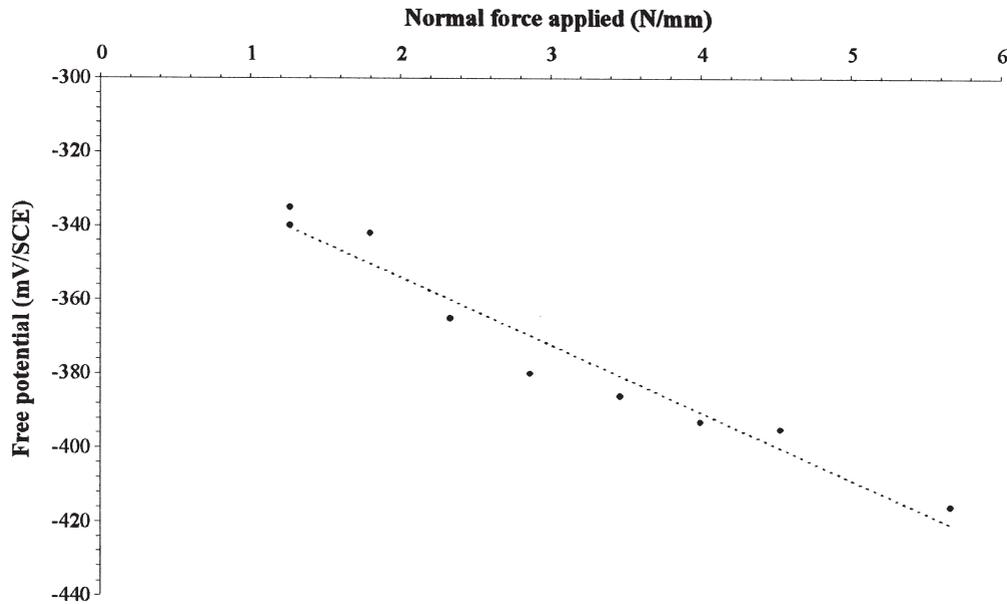
Fig. 7. Free corrosion potential at 10,000 cycles of fretting as a function of normal force applied. Contact PMMA Ø20/316L SS plane in Ringer's solution. Frequency 1 Hz, displacement  $\pm 40 \mu\text{m}$ .
