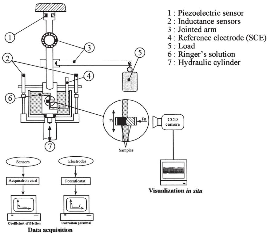
Fig. 2. Tribomines® fretting set-up.
