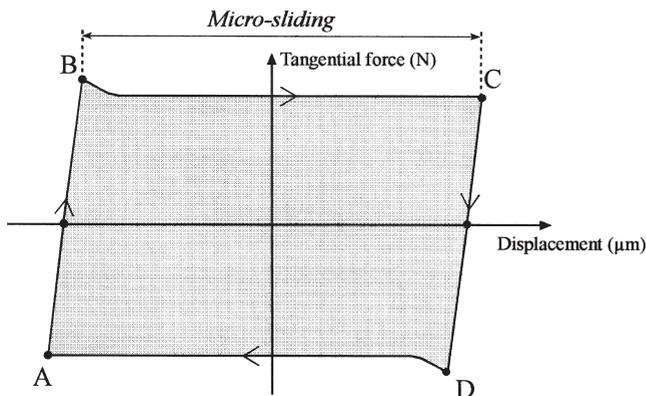
Fig. 8.  $F_T$ -D cycle used to calculate the interfacial energy dissipated.
