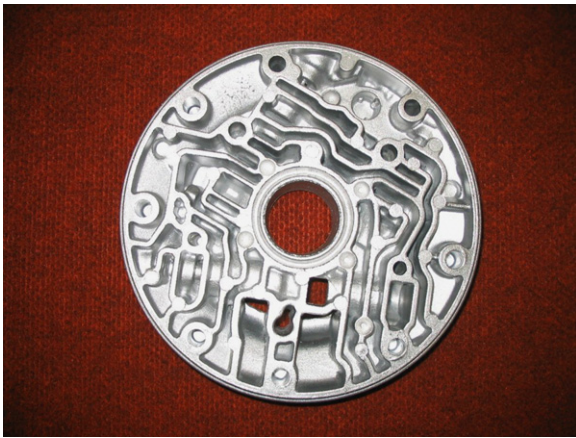
Fig. 2. The pump cover casting (~1700 g in weight, ~215 mm in diameter and 2–12 mm in thickness with alloy ADC12) made in an industrial die-casting machine with a vacuum system used.
