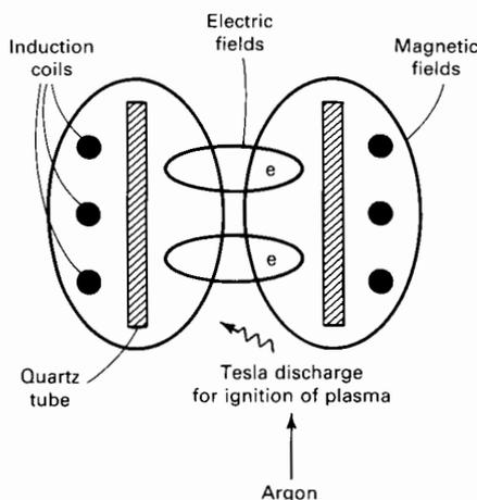
absorption could not match. The high-temperature and inert argon atmosphere of the plasma also greatly lessened the chemical and matrix interferences of flame emission techniques.
