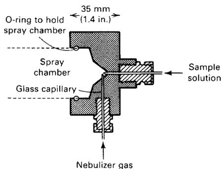
though these nebulizers perform well over extended times with dilute aqueous solutions, the fine dimensions of the sample capillary and the gas annulus make the nebulizer prone to blockage by small particles in the sample solution or the argon gas supply. Such blockages may stop sample and gas flows entirely or alter the flows, making detected signals erroneous in comparison to previous calibrations.
