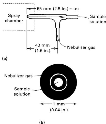
diameter droplets can be effectively desolvated, dissociated, atomized, and excited in the residence time of a few milliseconds in the plasma. Larger droplets contribute to excessively noisy analytical signals and cool the plasma by the introduction of too much water; they must be removed by passing the aerosol through a spray chamber after nebulization and before transport into the plasma by the carrier gas.
