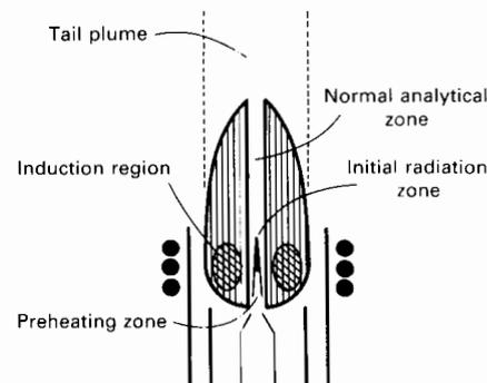
tion of varying wavelengths in the ultraviolet and visible portion of the spectrum is emitted on the nanosecond time scale as the electrons return to lower energy levels. The wavelength of this emitted radiation is characteristic of the atomic species present in the plasma and the intensity of the emitted radiation is proportional to the quantities of each atomic species present. Thus, analysis of the emitted radiation provides qualitative and quantitative elemental analysis.
