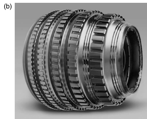
2.6 (a) A 2000 ton forge force inertia welder (model 2000B) and (b) a titanium low-pressure rotor assembly for an aero engine produced using the 2000 ton welder. (Courtesy of Manufacturing Technology, Inc.)
