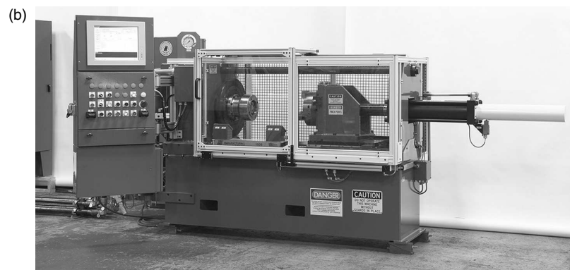
2.5 Typical IFW machines and products (a) 15 ton welder, (b) 40 ton welder, (c) light-weight piston for aircraft pump produced by the 15 ton welder and (d) turbine wheels produced by the 40 ton welder. (Courtesy of Manufacturing Technology, Inc.)
