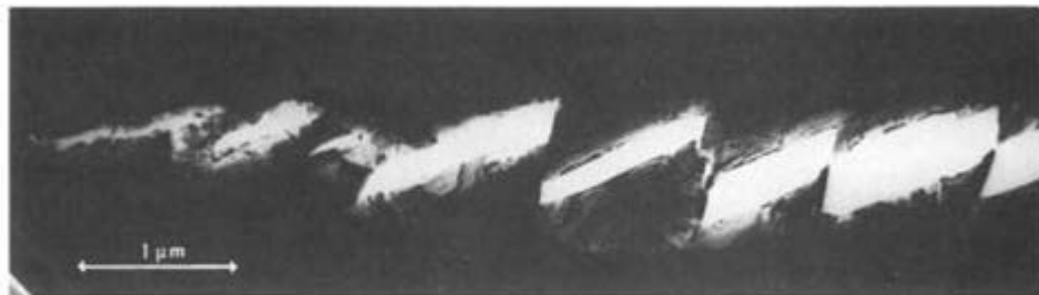
Fig. 8. Side view of a growing fracture in a thin film of gold. Holes are shown nucleating ahead of the crack; see LYLES and WILSDORF [1975]. (Courtesy H. G. F. WILDORF).
