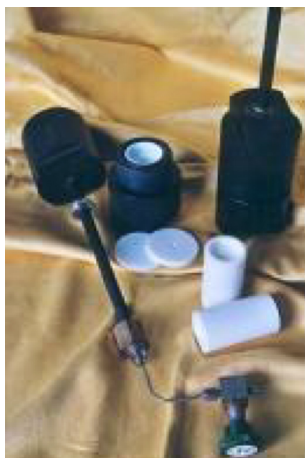
Fig. 2. Presentation of microwave autoclave reactor RAMO.
