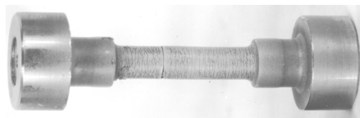
Fig. 7.44 Crack location on specimen surface with Co32Ni21Cr8AlY coating (liquid penetrant testing), 900 cycles
