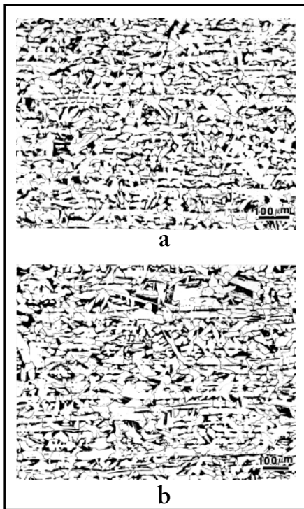
Fig. 2 The general microstructure of the (a) longitudinal and (b) transverse planes of the RMS Titanic plate. (4% picral + 2% nital etch — 100 \times )
