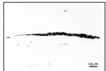
Fig. 5 View of a large silicate inclusion (dark gray) and smaller sulfides (light gray) of the RMS Titanic plate in the transverse plane. (Unetched — 100 \times . Reproduced with permission of the Iron & Steelmaker. [13] )
