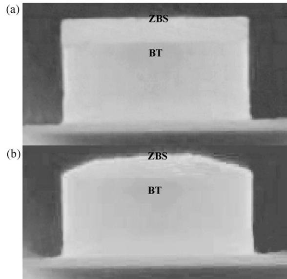
Fig. 2. Wetting behavior between ZBS glass and BaTiO<sub>3</sub> at 900 °C.
