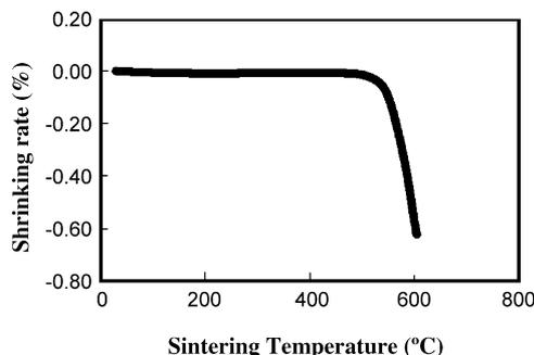
Fig. 1. Result of dilatometric analysis of ZBS glasses.
