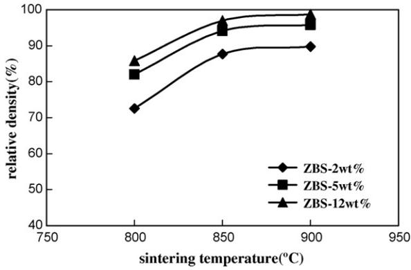
Fig. 4. Variation of the relative densities of the BaTiO<sub>3</sub> ceramics with the amount of glass addition and sintering temperature.
