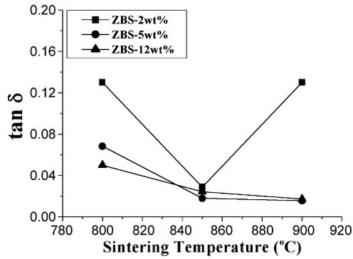
Fig. 7. Dielectric loss of the sample added with 5 wt% ZBS glass as a function of sintering temperature.
