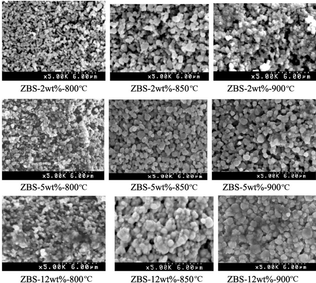
Fig. 5. Microstructure development of the samples with various amounts of added ZBS glass sintered in the 850–900 °C temperature regions.
