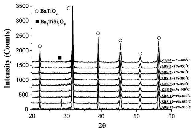
Fig. 3. XRD patterns of the samples with various amounts of added ZBS glass sintered in the 850–900 °C temperature regions.
