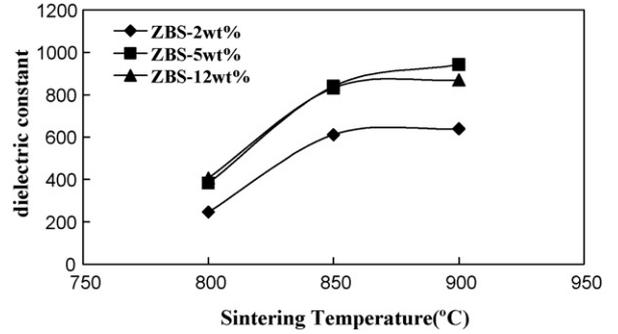
Fig. 6. Effects of the various amounts of added glass on the dielectric constant of BaTiO<sub>3</sub> ceramics.
