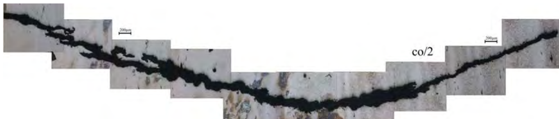
Fig. 5. Fusion-line cracks in the specimen that was welded by Co-base filler metal.
